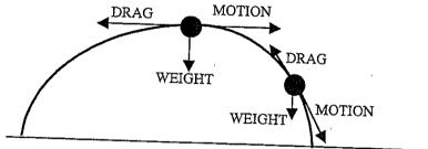
Factors causing air resistance to increase: area of ball, velocity, density of air, etc.
