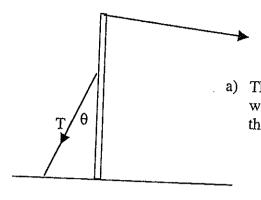
a) The clockwise torque about the base from the electric wire is balanced by the anticlockwise torque provided by the cable in the ground.
